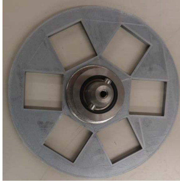
Figure 3.7. CT Specimen Polishing Jig
